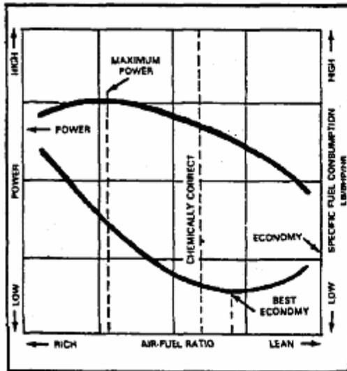
Fig. Note graph showing relationship of engine power, fuel consumption, and air-fuel ratio. Note how stoichiometric mixture or ideal mixture is between maximum power and best economy. (Ethyl Corporation)
