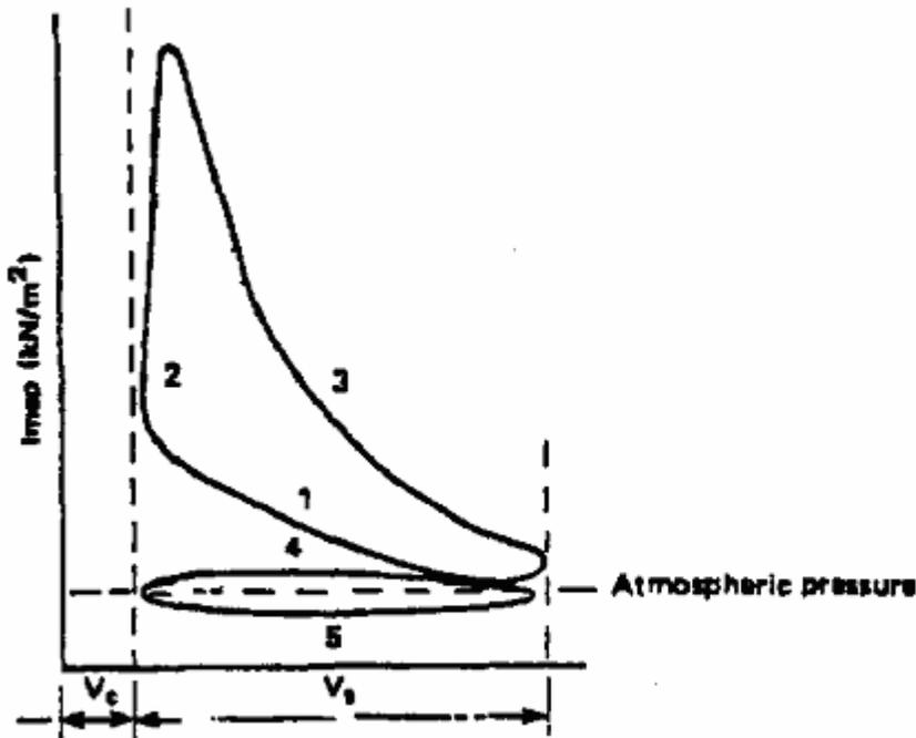
Fig. Pressure-volume indicator diagram. (1) compression, (2) combustion, (3) expansion, (4) exhaust, (5) induction.
