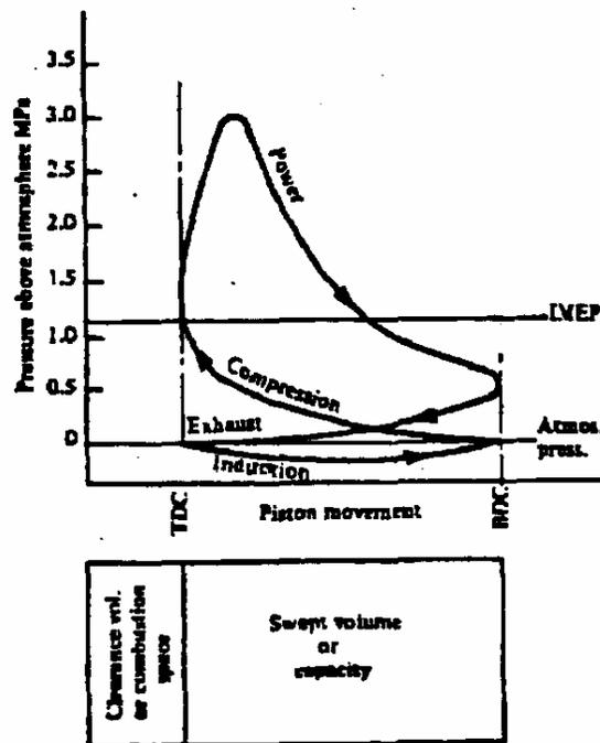
Figure Indicator diagram
