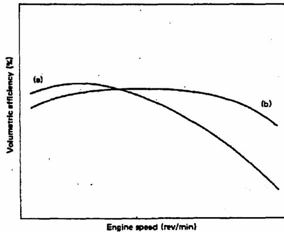
Fig. Volumetric efficiency and engine speed. (a) petrol engine, normally aspirated with carburettor. (b) compression ignition engine, normally aspirated.
