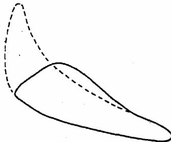
Fig. pV diagram: retarded ignition
