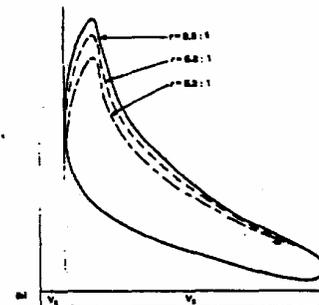
Fig. Petrol engine diagrams. (a) pCA diagram, (b) pV diagram.
