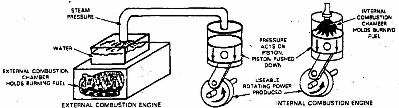
Fig. External combustion engine burns fuel outside cylinder. A steam engine is an external combustion engine. Internal combustion engine, like car engine, burns fuel inside cylinder.
