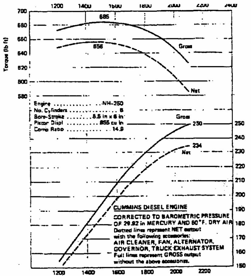
Figure A typical engine power curve.
