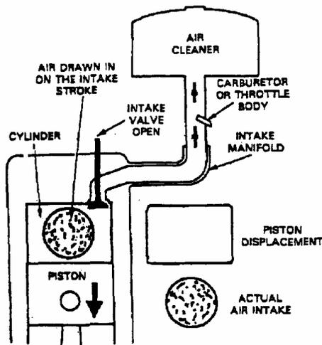
Fig. Volumetric efficiency is comparison of actual air intake and theoretical potential for air intake. (Deere & Co.)
