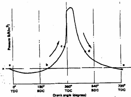
Fig. Rate of change of pressure diagram. (a) inlet valve commences to open, (b) inlet valve closes, (c) ignition commences, (d) exhaust valve opens, (e) exhaust valve closes. xx, atmospheric pressure.
