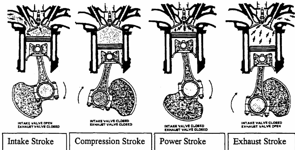
\* Intake (induction or inlet) stroke: The intake valve has opened. The piston is moving downward, drawing a mixture of air and gasoline vapor into the cylinder.
